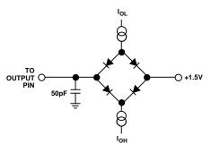
Figure 14. Equivalent Device Loading for AC Measurements (Including All Fixtures)
